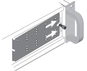
When properly installed, the security panel will still allow you to monitor all the channel status LED's and power LED. The amplifier front panel will look like the illustration, right, after installing the security plate.
